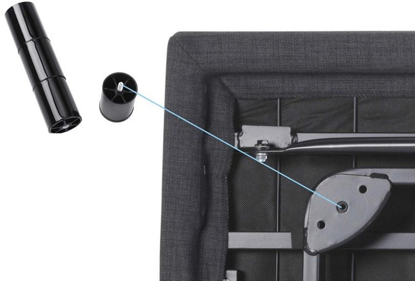
The legs must be installed onto the adjustable base; the base will not operate properly without them. Legs **MUST** be a **MINIMUM** of 6" to allow for articulating clearance. **IMPORTANT:** Using **ONLY** one 3" segment of the leg will result in damage to the base, void the warranty for improper use and may cause damage to the floor. Ensure all 6 legs are installed prior to use.
